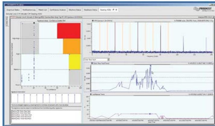
*Fig. 7: This plot shows a low confidence factor despite of high band amplitude. This means that these amplitudes do not belong to the failure represented by the bands in the upper spectrum since only a few peaks match with this failure pattern.*
