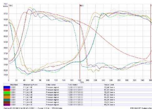
*Fig. 4: Dynamic pressure curves for all 4 cylinders over one full revolution, clearly pointing to a damaged discharge valve*
