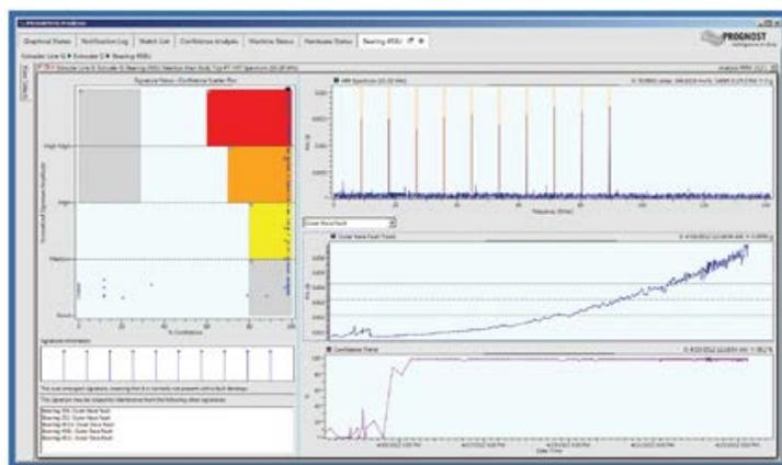
*Fig. 8: This plot shows a high confidence factor and high band amplitude which result in an alarm. All bands show matching peaks inside.*
