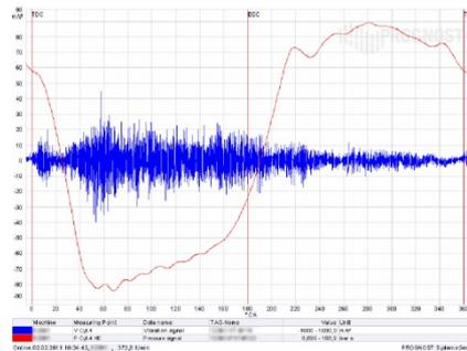
*Fig. 3: Time signals for one revolution showing vibration acceleration and dynamic pressure of a reciprocating compressor cylinder*
