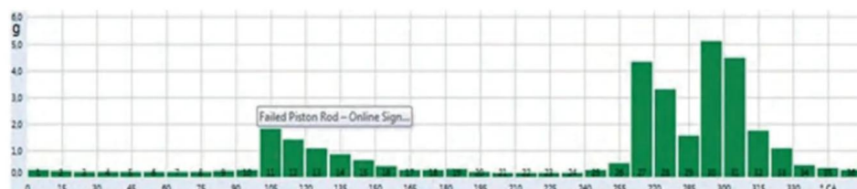
FIGURE 11 Bad Condition 0 - 7 kHz RMS 36 segmented analysis.
