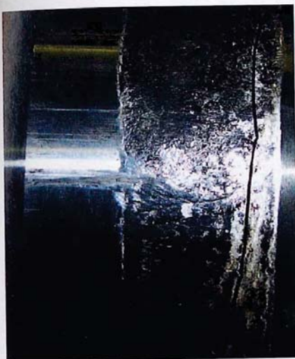
■ The piston rod with a 75% circumferential crack.
