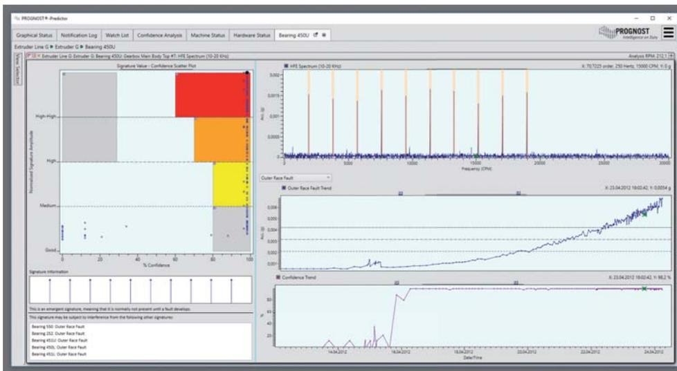
*High Confidence Factor and high band amplitude: This condition results in an alarm and the component being identified in red color.*
