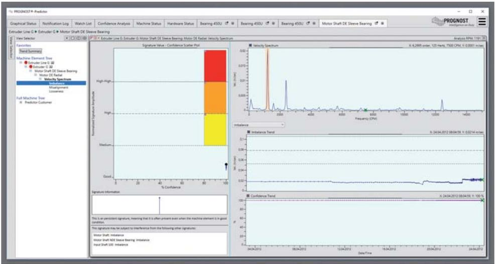
Detection of imbalance failure pattern with trending of the Confidence
