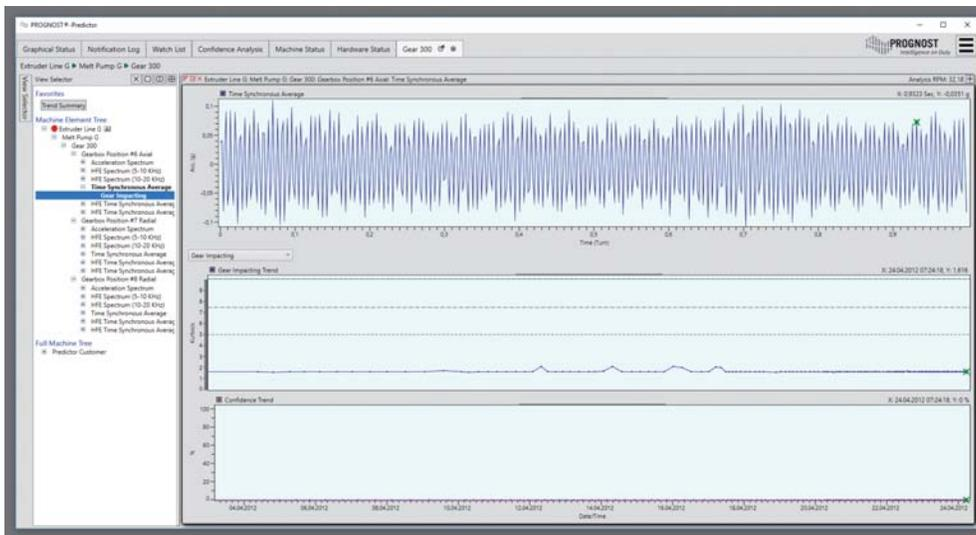
Gear Imaging isolates the vibration generated by each gear in the gearbox while rejecting interfering vibration. Damage to an individual tooth will produce localized high-amplitude peaks.
