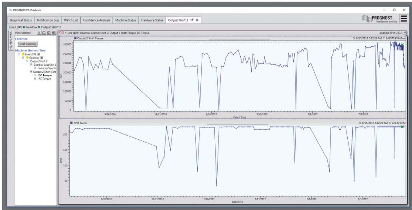
Trend plots of output shaft torque (above) and machine speed (below). Critical torque events are clearly visible.
